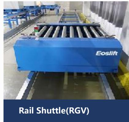
**Features:** Widely used in the logistics system: fast speed, low cost, all in a limited space to achieve reciprocating movement.
