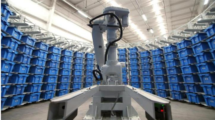
Robot material box type automatic warehouse (MiniLoad) for container storage unit. The robot manipulator in a container 360° rotating annular ring. Sorted goods located at the mouth of roadway, takes out the goods or ships to tunnel mouth. The entire solution mainly solves problems of secondary caching and multi-category selection in e-commerce and other industries.
